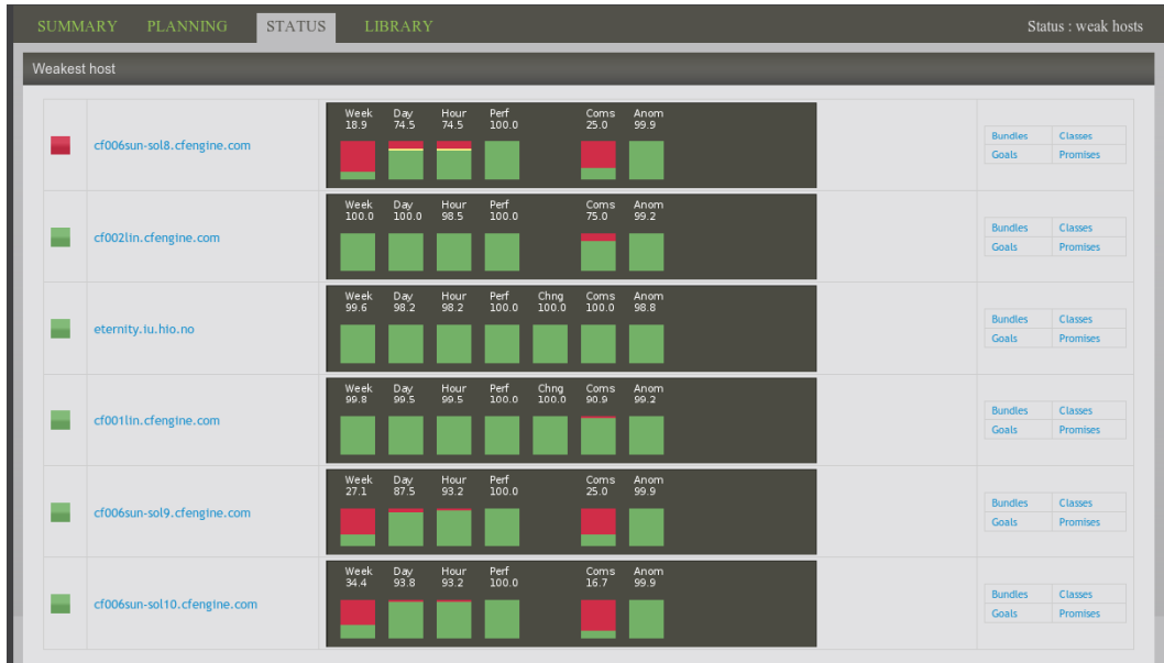
Weakest hosts broken down by compliance, performance and change.
