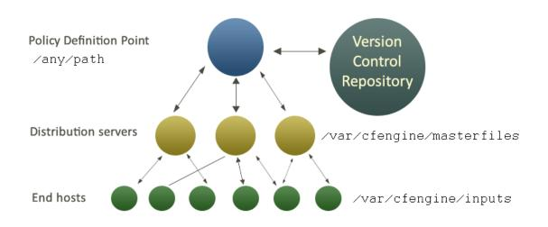
The figure below shows how decisions flow through the parts of a system.
